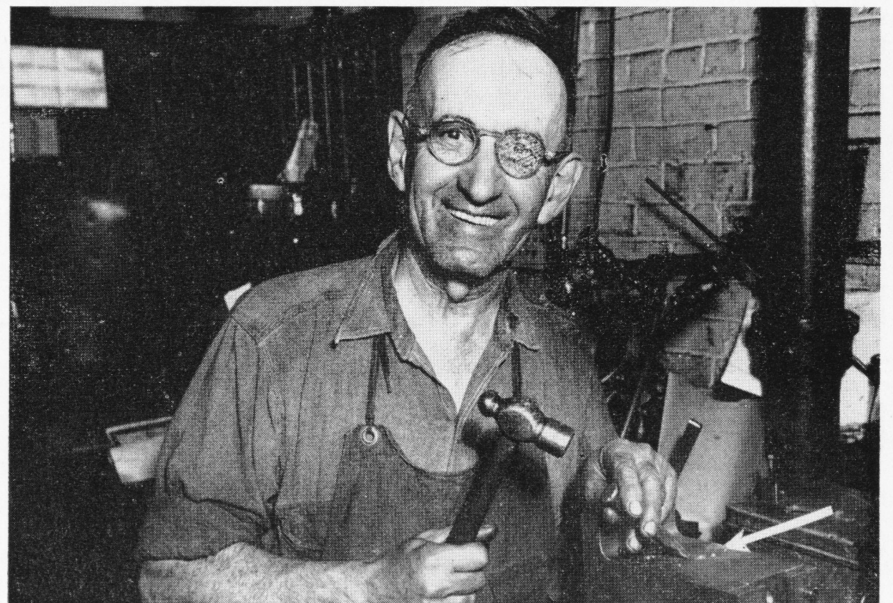
Barney Dougherty, of the West Machine Room, wears the prescription safety glasses which saved one of his eyes when a piece of steel suddenly flew—with terrific force like shrapnel—from a broken tap which he was attempting to remove, as he demonstrates in the above picture.
